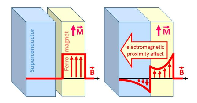
Sketch of the magnetic effects the superconductor-ferromagnet bilayer has both when the layers are separated from each other and when they are put in contact. Credit: Sergey Mironov
