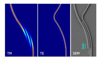
A scanning electron micrograph (right) of the three-waveguide polarization beam splitter, and the light intensity of the two polarization components (TE/TM). Credit: A\*STAR Institute of High Performance Computing
