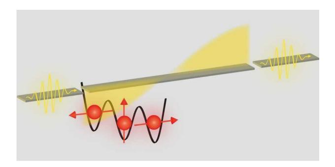
A spin-trio of electrons trapped in quantum dots (red). Quantum mechanical tunnelling between the quantum dots results in a dipole moment that couples strongly to the electromagnetic wave of a resonator (yellow). Credit: Visualisations: ETH Zurich / Andreas Landig
