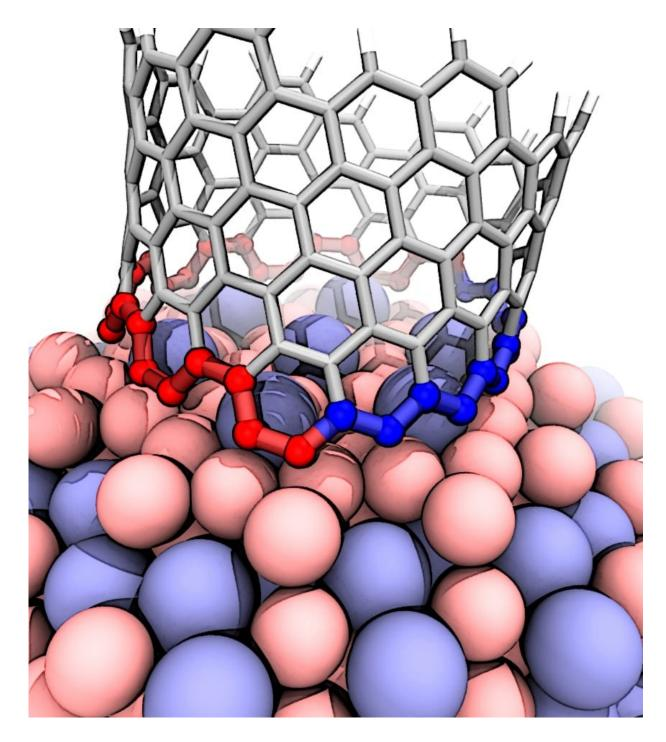
This illustration shows the interface between a growing carbon nanotube and a cobalt-tungsten catalyst. The atomic arrangement of the catalyst forces the nanotube to quickly transition from zigzag (blue) to armchair (red), which ultimately grows a nanotube that's neither one nor the other, but nearly in the middle. The transition is a previously undiscovered characteristic of carbon
