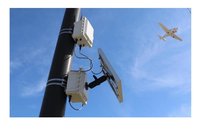
A plane flies over the Blueavion f1 data collection technology at the Purdue University Airport. The device uses data collection technology to help small airports improve operations data collection. The technology was developed at Purdue University and is available through Bluemac Analytics. Credit: Darcy Bullock, Purdue University
