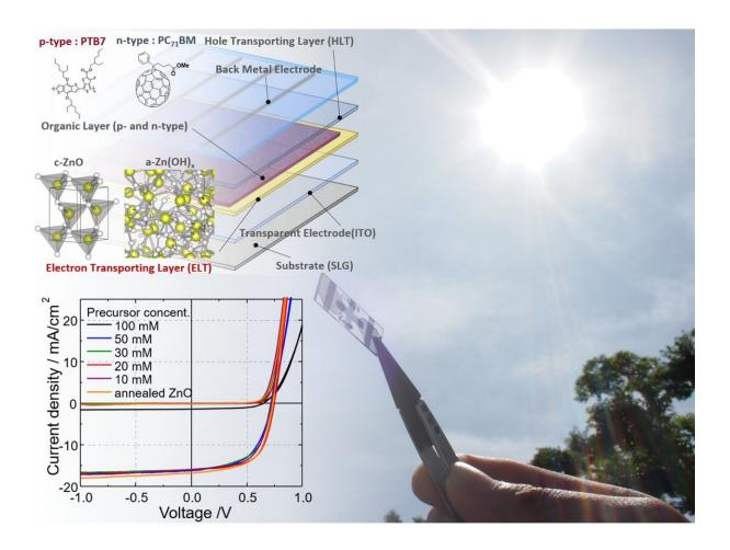
Figure: Organic photo voltaic solar cells and schematic figure of the cell structure. Current density voltage (JV) characteristics during light irradiation and dark condition. Credit: Osaka University
