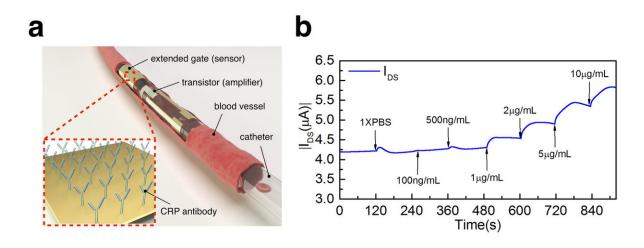
Figure 1 a) Conceptual image of a CRP sensor in ventricular catheter implanted in blood vessel. b) Transistor channel current increase against CRP concentration. Credit: @The University of Hong Kong
