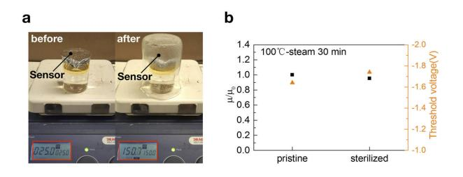
Figure 2 a) Photograph of OFET device before and during 100 ?-saturated steam sterilization. b) Normalized mobility and threshold voltage change after 30 minutes' saturated steam sterilization. Credit: @The University of Hong Kong
