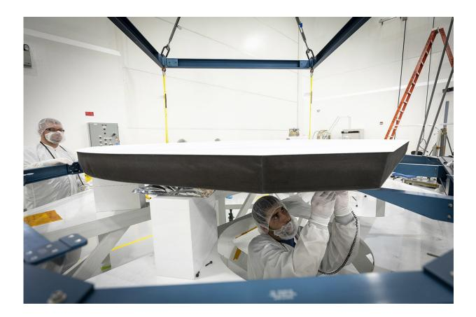
Parker Solar Probe's heat shield is made of two panels of superheated carboncarbon composite sandwiching a lightweight 4.5-inch-thick carbon foam core. To reflect as much of the Sun's energy away from the spacecraft as possible, the Sun-facing side of the heat shield is also sprayed with a specially formulated white coating. Credit: NASA/Johns Hopkins APL/Ed Whitman
