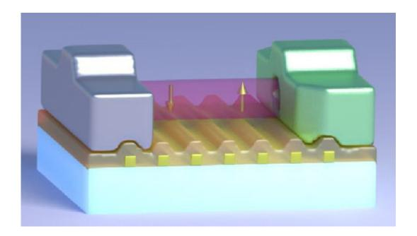
3-D model of the Yu-Shiba-Rusinov device. Two electron spins are defined along the nanowire, by placing appropriate voltages on the tiny electrodes under the nanowire. By coupling the spins to the superconductor Yu-Shiba-Rusinov states can be realized. Observation of these states are achieved by analyzing the current through the device from the normal metal to the superconductor. Credit: Niels Bohr Institute
