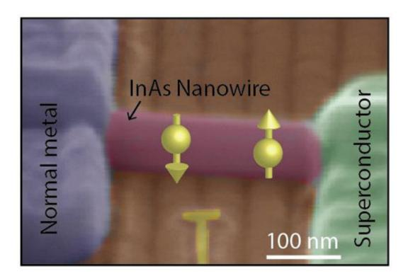
Scanning electron microscope micrograph of a semiconductor nanowire, made from Indium Arsenide, connected electrically to a superconductor and a normal metal. The location on the nanowire of the two spins - the microscopic magnets are illustrated by the arrows. In this case the microscopic magnets are created by electron spins. Credit: Niels Bohr Institute
