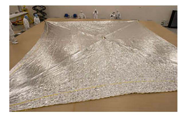
The solar sails attached to NASA's Near-Earth Asteroid Scout were tested in June in a clean-room at NeXolve Corp. in Huntsville, Ala. RIT professor Grover Swartzlander and mechanical engineering undergraduate Amber Dubill, a student leader in RIT's Space Exploration research group, attended the test deployment. Credit: NASA/Emmett Given
