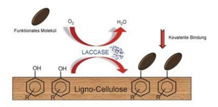
How laccase alters the surface of the wood: A desired molecule is bound to the cellulose in the wood chemically with the aid of the enzyme. Credit: Empa
