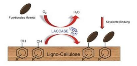
How laccase alters the surface of the wood: A desired molecule is bound to the cellulose in the wood chemically with the aid of the enzyme. Credit: Empa
