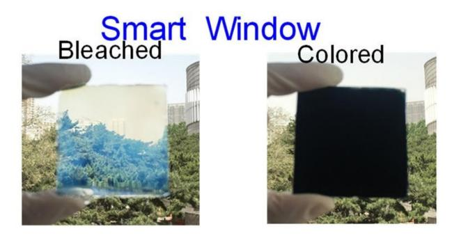
Photographs showing one of the three properties of the sterile smart window: control of visible light transmission. Credit: Xu et al. ©2018 American Chemical Society
