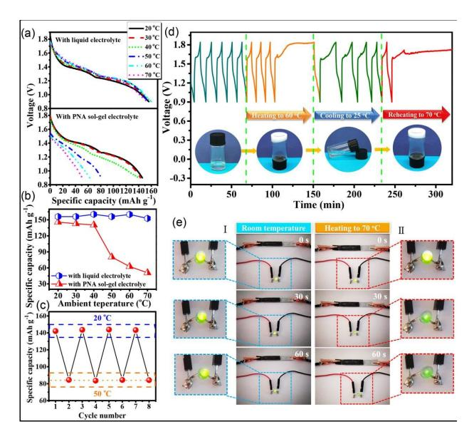
Dynamic electrochemical performance the thermoresponsive  $Zn/\alpha$ -MnO2 batteries at different temperature. Credit: ©Science China Press
