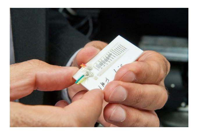
Scientists at UConn and the United Technologies Research Center used direct write technology, an advanced form of additive manufacturing, to create a novel sensor that can be embedded into machine components while they are being made. The sensors can detect and report wear and damage to a part to the machine's user. Credit: Peter Morenus/UConn
