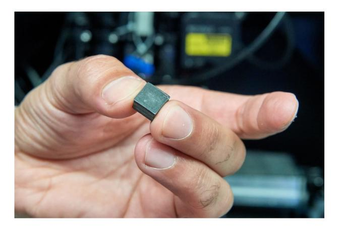
Scientists at the United Technologies Research Center and UConn used an advanced additive manufacturing technique called Direct Write to make customized 3D-printed magnets of unique shapes. These magnetic materials can make machine designs more efficient and lighter. Credit: Peter Morenus/UConn
