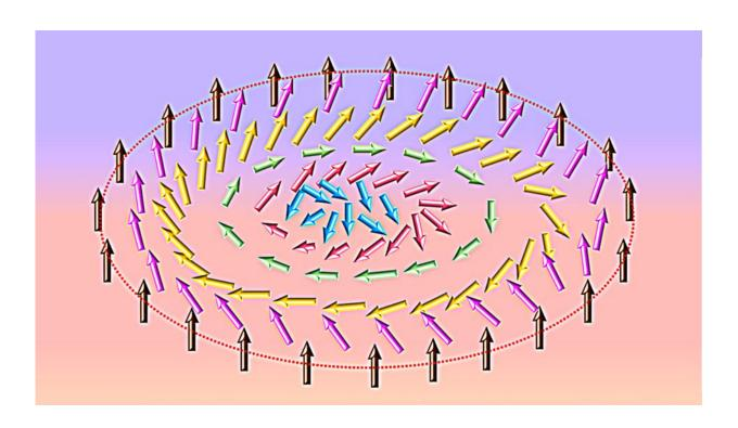
An illustration of the magnetic vortex, known as a skyrmion, that could star in the next generation of digital memory. Each arrow indicates the direction of the magnetic axis in an individual atom. Credit: Nanoscale / Royal Society of Chemistry
