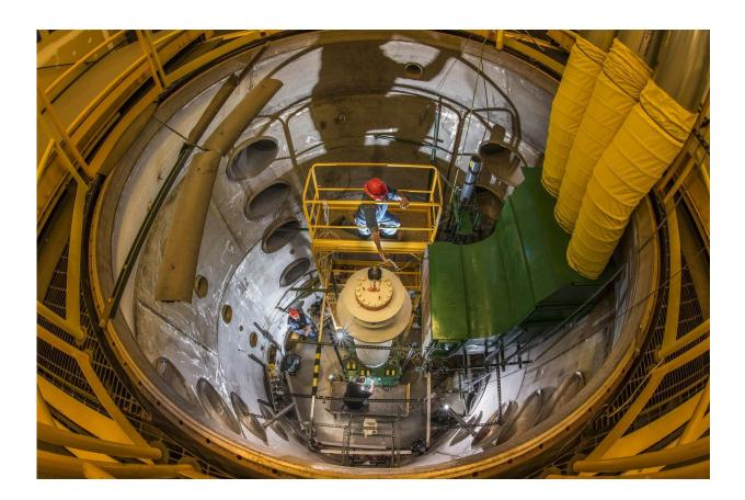
Sandia National Laboratories designed and constructed a dry-cask simulator for boiling water reactor assemblies to study how hot spent nuclear fuel will get during storage and how the fuel's peak temperatures affect the integrity of the cask over time. Electrical heaters shaped like fuel rods were used instead of spent nuclear fuel in the otherwise prototypical fuel assembly. Credit: Randy Montoya
