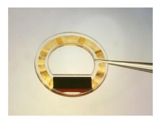
Encapsulated sensor implant for measuring intraocular pressure. Credit: Fraunhofer IMS
