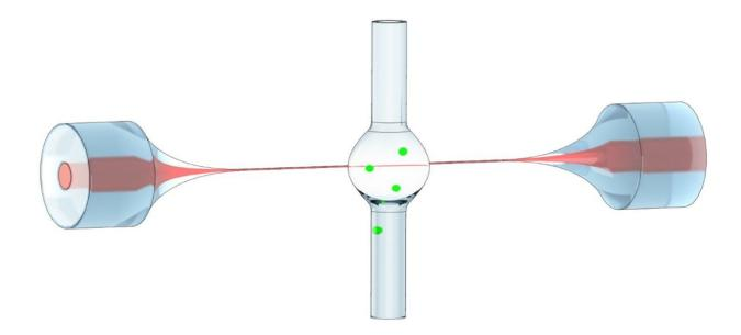
A diagram showing the new WGR experiments. Test particles (shown here in green) are passed through a light field, which distorts the light wavelength, which can be used to detect the particles. Credit: Okinawa Institute of Science and Technology
