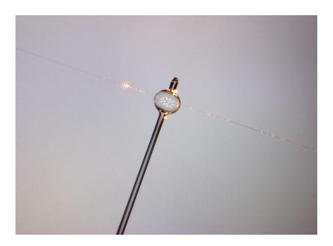
A magnified photograph of a glass Whispering Gallery Resonator. The bubble is extremely small, less than the width of a human hair. Credit: Okinawa Institute of Science and Technology
