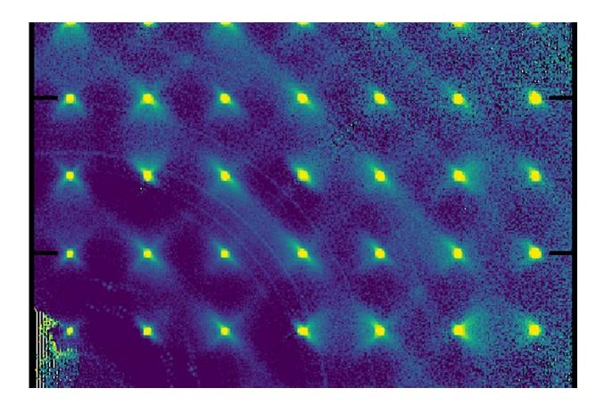
This shows the asymmetry of the butterfly-shaped scattering, which Argonne scientists found was strongly correlated with piezoelectric behavior. Credit: Argonne National Laboratory
