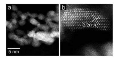
Analysis using high-angle annular dark-field scanning transmission electron microscopy (HAADF-STEM) revealed: (a) small and flat ruthenium patches over a large domain and (b) the lattice spacing corresponding to that of facecentered-cubic ruthenium nanoparticles. Credit: Chemical Science
