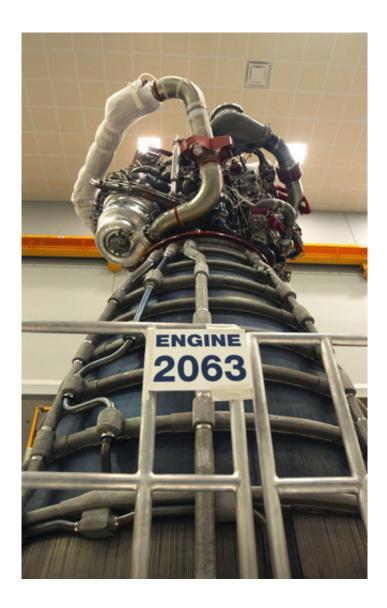
An AR-22 engine, being used for a developmental reusable spacecraft, is seen in Stennis, Miss., Monday, July 2, 2018. Triggering a massive cloud of vapor and a roar, officials on Monday test fired the rocket engine designed to be part of a reusable spacecraft that can launch into space repeatedly with a quick turnaround time. (AP Photo/Gerald Herbert)
