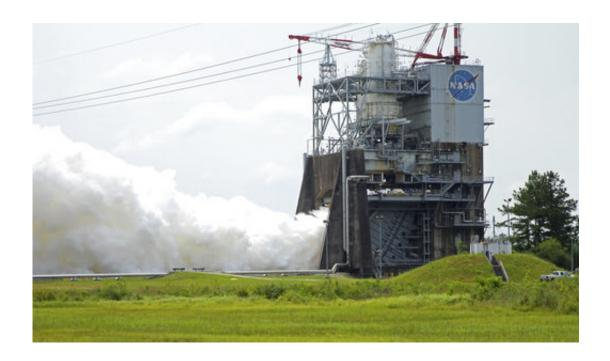
An AR-22 rocket engine is test fired on the A-2 test stand at the NASA Stennis Space Center in Stennis, Miss., Monday, July 2, 2018. Triggering a massive cloud of vapor and a roar, officials on Monday test fired the rocket engine designed to be part of a reusable spacecraft that can launch into space repeatedly with a quick turnaround time. (AP Photo/Gerald Herbert)
