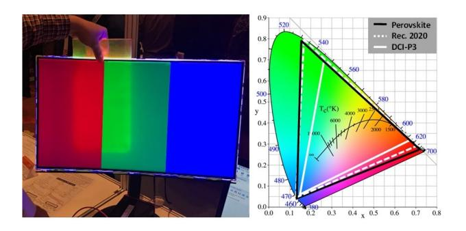
(Left) Photo showing the colour-enhancement effect from using a prototype of the perovskite-based film. When the film is placed between the backlight unit and the display screen, a spectrally "purer" red and green colour is observed. (Right) Figure showing the coverage of the colour space by perovskite, compared to Rec. 2020 and DCI-P3 colour standards. Credit: National University of Singapore
