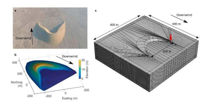
Barchan dune geometry, in reality and the simulations. (a) Image of an isolated Qatari barchan dune from an aerial drone, courtesy of Sylvain Michel. (b) Elevation profile of the same barchan, from data courtesy of Michel Louge. (c) Mesh generated model of the same dune. The red arrow indicates the location of the point force for the simulation in the video. Credit: GeoSpace
