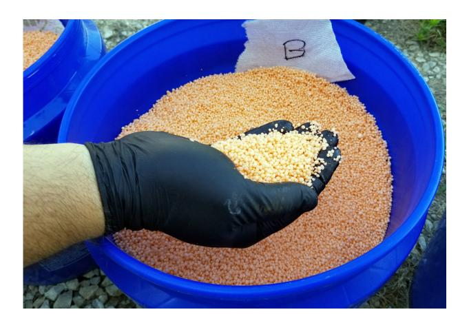
Urea granules treated with Nutrisphere-N maleic-itaconic acid polymers (MIPs). Credit: Darin Lickfeld
