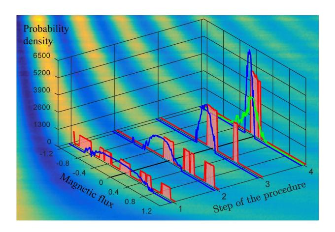
Probability distributions (shown in red and blue for the two algorithms used in the work) narrow down in consecutive steps of the algorithms, leading to the precise identification of the magnetic-flux value. The green curve is the standard-quantum-limit distribution and the background is the interference pattern characteristic of the device. Credit: Sergey Danilin and Sorin Paraoanu, Aalto University, with data from the paper doi: 10.1038/s41534-018-0078-y
