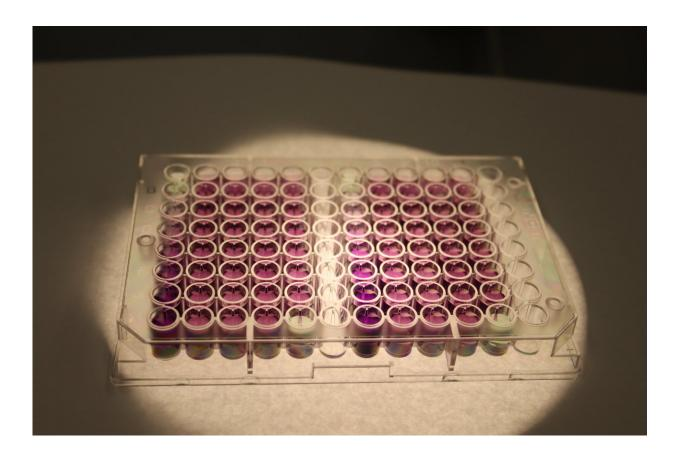
Soil protein is measured in the lab using a color-reading process called colorimetric analysis. Credit: Steve W. Culman
