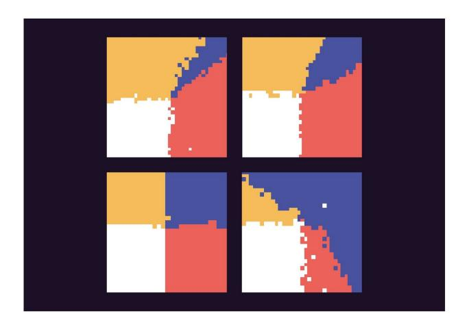
Phase diagrams showing the four different regions observed in the experiment: white -- superfluid without photons; red and yellow -- photons in only one of the cavities; blue -- photons in both cavities simultaneously (mixed phase). As the coupling between the orders is increased, the mixed-phase regime (blue) becomes increasingly favourable. Credit: Esslinger group, ETH Zurich (adapted from doi: 10.1038/s41563-018-0118-1)
