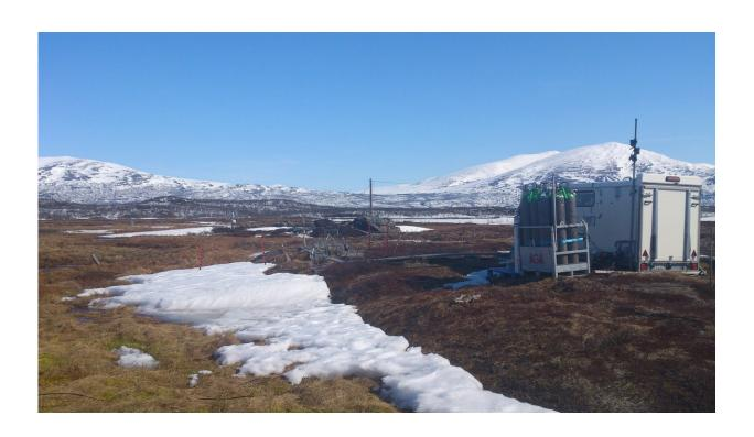
Stordalen Mire study site. The biogeochemistry hut is connected to autochambers, allowing measurements of gas flux. Credit: Caitlin Singleton
