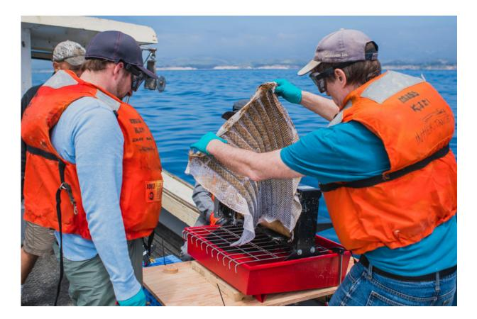
In recent open-water tests, Oleo Sponge worked just as researchers had predicted: It was able to successfully remove oil sheen from the surface of the water, leaving no visible trace behind. Credit: Argonne National Laboratory
