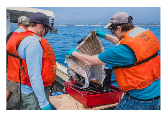
In recent open-water tests, Oleo Sponge worked just as researchers had predicted: It was able to successfully remove oil sheen from the surface of the water, leaving no visible trace behind. Credit: Argonne National Laboratory
