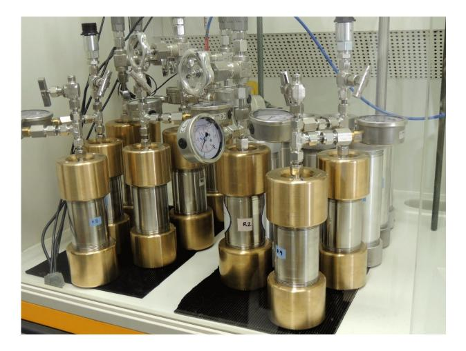
High pressure reactors at the Hamburg University of Technology (TUHH) simulated deep-sea conditions of biodegradation. Results from the experiments were shipped to Penn State University for chemical analysis. Credit: C-IMAGE Consortium
