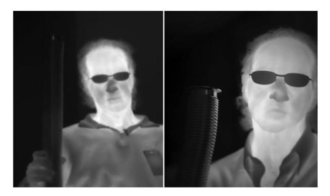
The image on the right shows the improved resolution of the Strained-Layer Superlattice, or SLS, detector array as compared with that of the Quantum Well Infrared Photodetector technology at left. Credit: NASA
