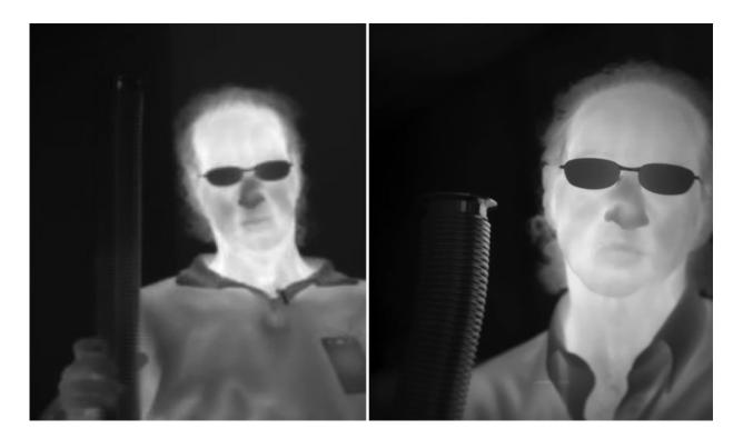
The image on the right shows the improved resolution of the Strained-Layer Superlattice, or SLS, detector array as compared with that of the Quantum Well Infrared Photodetector technology at left. Credit: NASA
