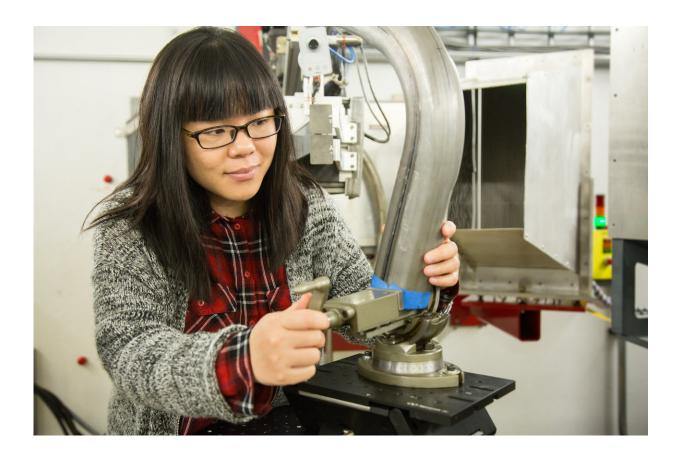
Lu Huang, USS industrial research engineer prepares a lightweighted advanced high strength steel component for neutron research at the Spallation Neutron Source's VULCAN instrument. Data from this study may make it faster and easier for companies to design automotive components that are lighter, more durable, and safer. Credit: ORNL/Genevieve Martin
