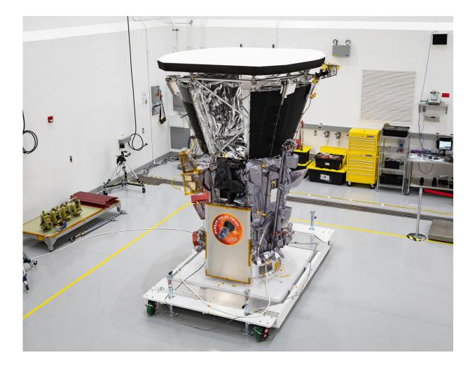
A Sun-skimming mission like Parker Solar Probe has been a dream of scientists for decades, but only recently has the needed technology -- like the heat shield, solar array cooling system, and fault management system -- been available to make such a mission a reality. Credit: NASA/Johns Hopkins APL/Ed Whitman
