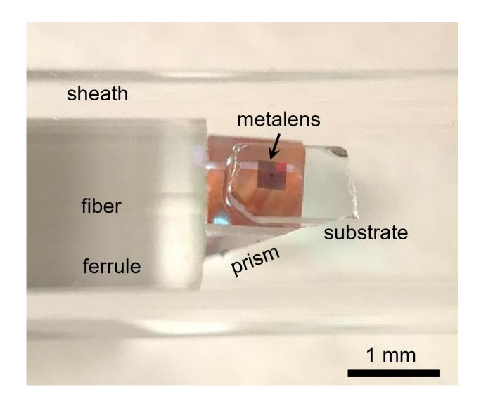
Researchers adopt metalens technology in a new endoscopic optical imaging catheter to better detect disease, including cancer Credit: Harvard University/Massachusetts General Hospital
