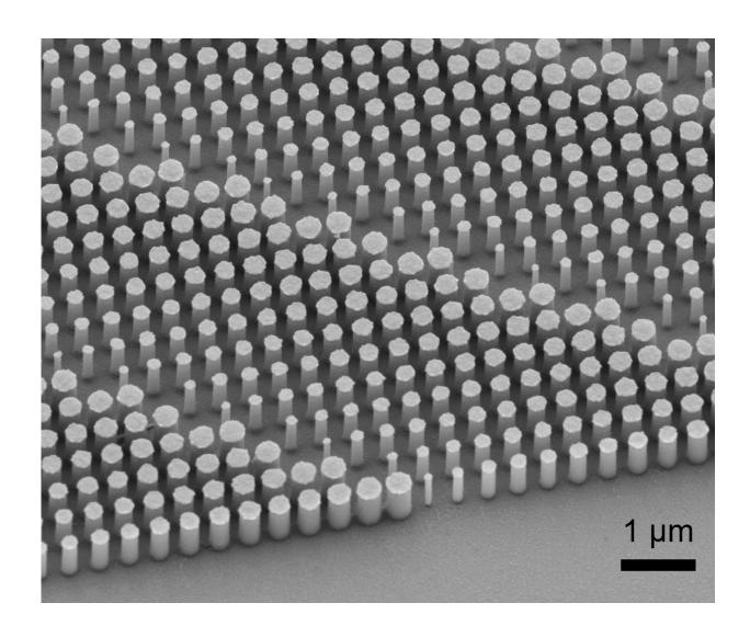
Scanning electron micrograph image of a portion of a fabricated metalens. Credit: Harvard SEAS
