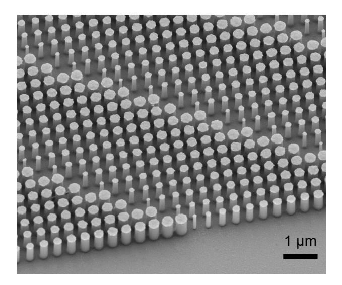
Scanning electron micrograph image of a portion of a fabricated metalens. Credit: Harvard SEAS
