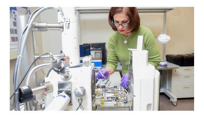
Afsaneh Rabiei is pictured here with the device she developed that can capture scanning electron microscopy (SEM) images in real time at temperatures up to 1,000 degrees Celsius while applying stresses as high as two gigapascal. Credit: North Carolina State University
