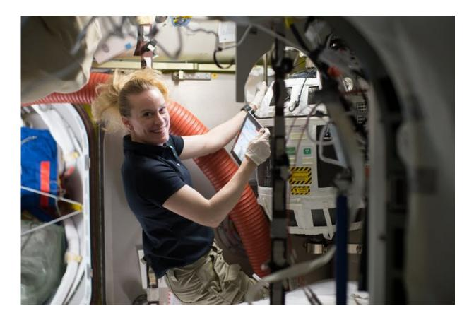
NASA astronaut Kate Rubins works with a Nitrogen/Oxygen Recharge System tank aboard the International Space Station. The tanks are designed to be plugged into the station's existing air supply network to refill the crew's breathable air supply. Credit: NASA
