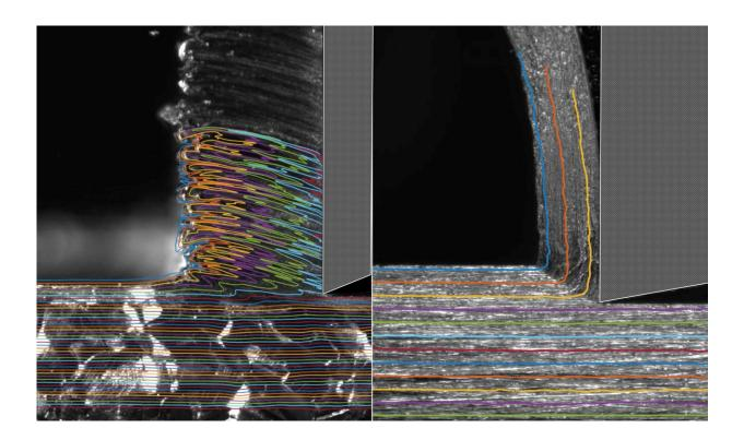
Purdue researchers have discovered a simple solution for cutting soft gummy metals (left) just as cleanly and easily as hard metals (right). Credit: Purdue University image/Anirudh Udupa
