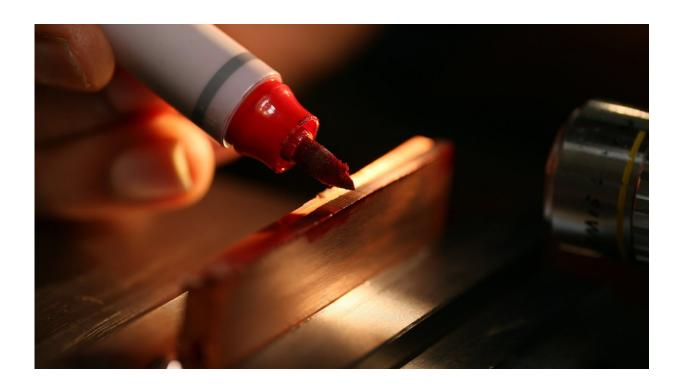
The application of a permanent marker, glue or tape makes gummy metals such as aluminum, stainless steels, copper and tantalum much easier to cut for industrial applications. Credit: Purdue University image/Erin Easterling
