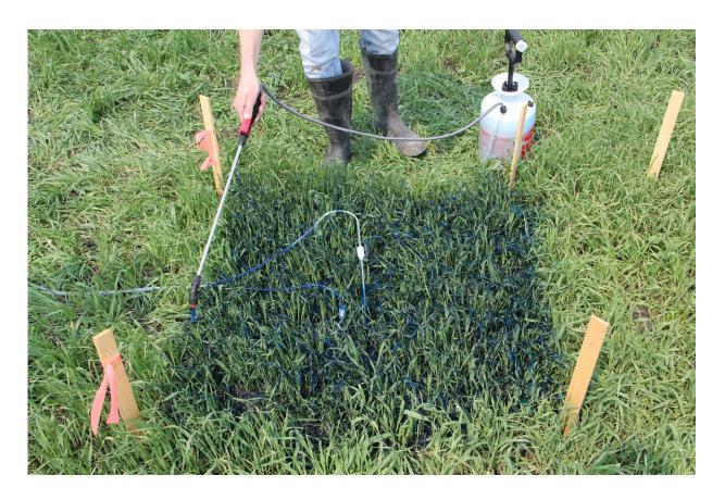
At the onset of the experiment, a pesticide sprayer is used to apply blue-dyed water on top of a 39 inch square (1 m by 1 m) soil plot. Credit: Genevieve Ali
