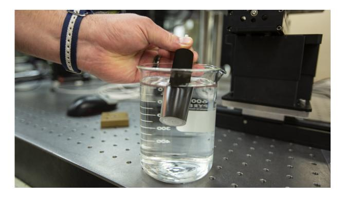
A metal sample modified to mimic shark skin repels water as it is placed in a beaker. The modified metal may some day be used to create submersibles that can travel more efficiently through water. Credit: Troy Fedderson | University Communication
