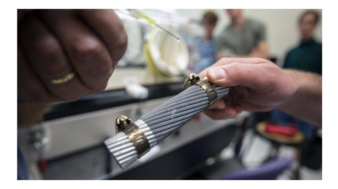
Blurred water droplets roll off of a section of wire used to transmit electricity. Dennis Alexander's lab is pursuing a project that will modify power line wires so that they repel precipitation. The work shows promise in reducing ice formation on power lines. Credit: University of Nebraska-Lincoln
