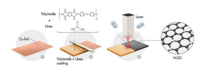
Laser treatment of a polymer coating on copper creates nitrogen-doped laserscribed graphene (NLSG) for use as a sodium-ion battery anode. Credit: Wiley-VCH Verlag GmbH & Co. KGaA. Image created by Xavier Pita
