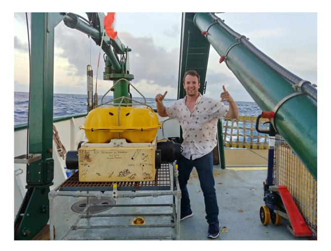
Blank poses with the last of 12 ocean-bottom seismometers to be placed off the southeastern shore of the Big Island of Hawaii in July. The seismic instruments are expected to capture information for the next two months about ongoing earthquakes and aftershocks associated with the eruption of Kilauea. Credit: David Blank
