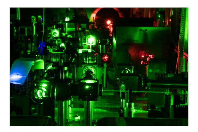
ISOLDE's resonant ionization laser ion source (RILIS) provided the first beams of neutron-rich chromium isotopes to the ISOLTRAP precision balance. Credit: Noemí Carabán González/CERN
