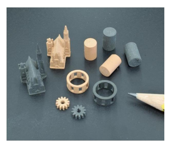
3-D printed ceramic items produced from simulated lunar regolith by Lithoz in Austria, a member of the URBAN consortium investigating 3-D printing for a lunar base. The grey items are 'green' items that have not been sintered (baked) while the light brown items have been sintered. Credit: European Space Agency
