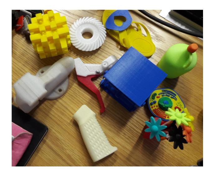
Sample items 3-D printed in high-performance polymers, produced by a prototype printer designed to operate in weightless conditions, designed by a consortium led by German aerospace company OHB System AG with Portuguese 3-D printing specialist company BEEVeryCreative. Credit: European
