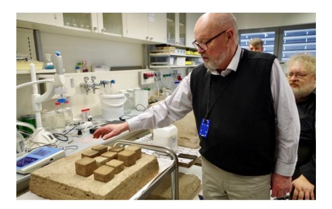
After determining the humic and fulvic acid content in peat and conducting the XRD analysis of elements and minerals, the possible test mixtures were modeled and small test pieces printed. On the photo, Toomas Tenno is showing these test pieces. Credit: Merilyn Merisalu
