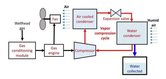
By using flared gas to power refrigeration, water can be harvested from the air. Credit: Vaibhav Bahadur
