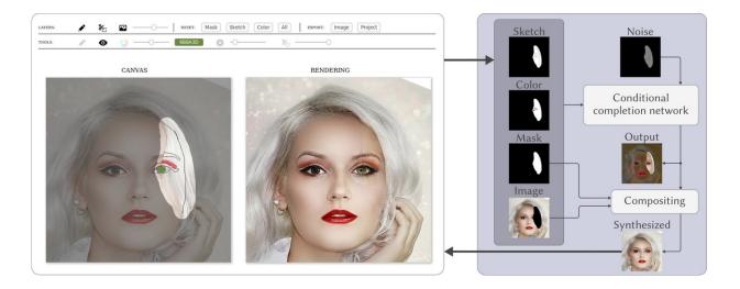
Faceshop consists of a web-based user interface (left) that enables a user to specify a region to be edited. Moreover, the user can draw strokes and color scribbles to guide the editing process. The core of the back end (right) is a deep image completion network that takes the user input and the original image to synthesize the edited result. Credit: Tiziano Protenier
