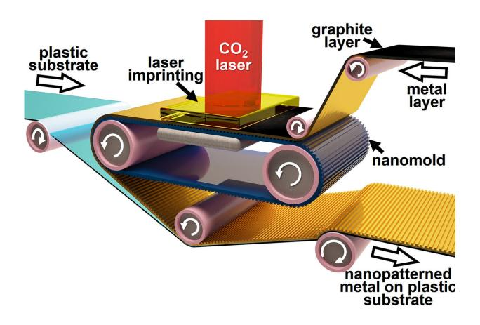
Roll-to-roll laser-induced superplasticity, a new fabrication method, prints metals at the nanoscale needed for making electronic devices ultrafast. Credit: Purdue University image/Ramses Martinez
