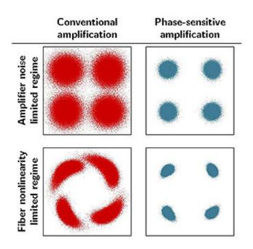
Signal constellation diagrams comparing conventional amplification and phasesensitive amplification in an amplifier noise limited regime (-2 dBm launch power) and a fibre nonlinearity limited regime (8 dBm launch power). Credit: Samuel Olsson
