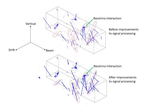
The latest improvements in MicroBooNE Time Projection Chamber (TPC) signal processing result in more completely reconstructed 3D particle tracks (bottom) than earlier techniques (top), which left gaps in the 3D images (see red circled areas for comparison). The improvement is crucial for distinguishing neutrino interaction signals (circled in green) from background signals generated by cosmic rays interacting with the fluid in the TPC. Credit: Brookhaven National Laboratory
