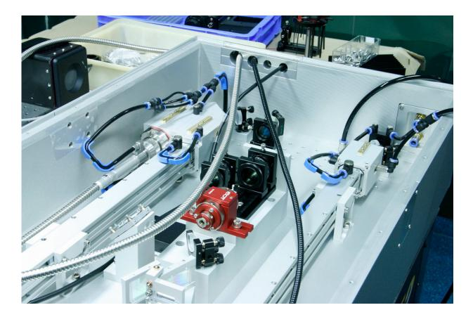
Main amplifier stages of the fiber laser system, where high pulse energies are generated. Credit: Fraunhofer IOF, Marco Plötner, Walter Oppel
